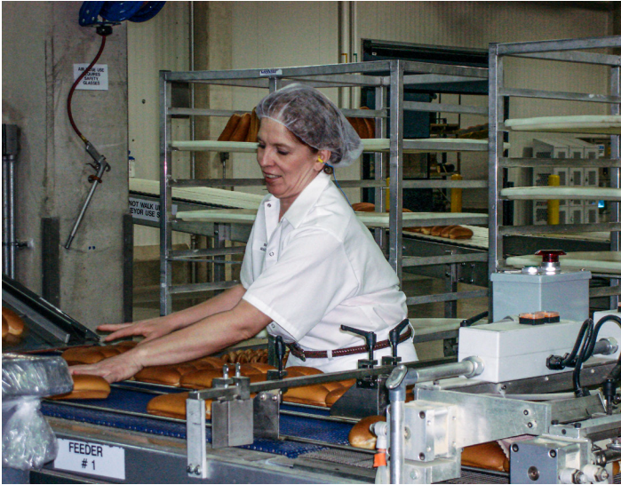
"Direct-Contact" application using oil free compressed air to blow-off crumbs in a commercial bakery.
