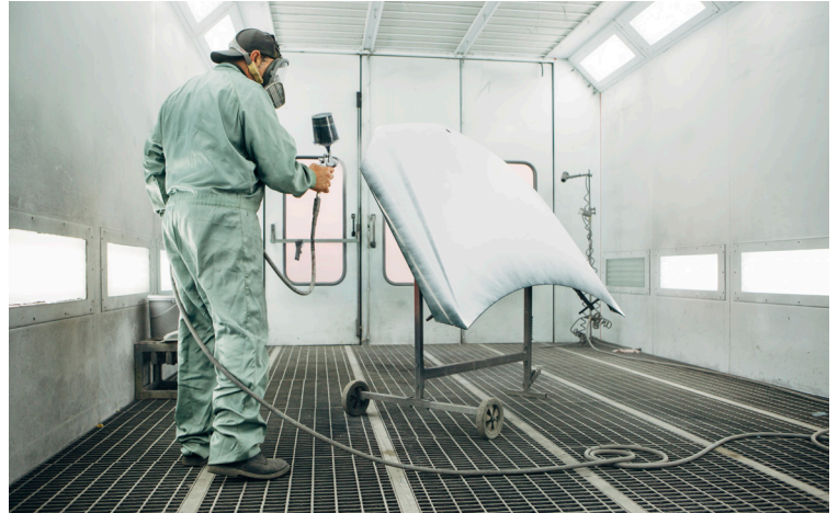
Oil free compressed air ensures a perfect paint surface
